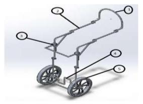
It is a lift frame that provides a mechanically adjustable support structure for restraint and skeletal support for an animal. This device was very helpful for animals recovering from injury or surgery. This model was light and versatile to facilitate use by the user a one-piece design making it simple to use while assisting the animal to walk or manoeuvre during the rehabilitation process.
